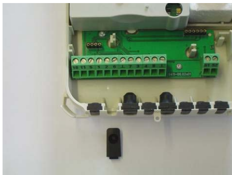
Figure 7: Open terminal block, one of the preshaped rubber parts removed
