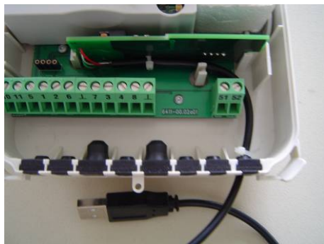
Picture 6: USB plug-in unit 68504688 in calculator housing 2
